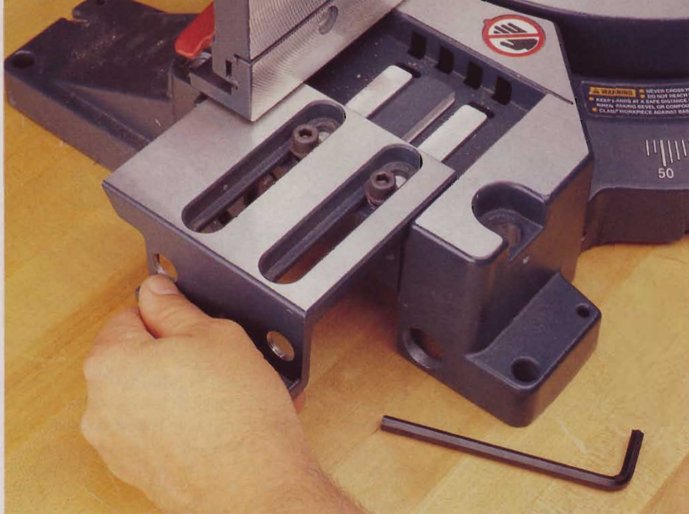
Above: Bosch's left extension table slides out for support and in for transport. The hex wrench stores on the base.
